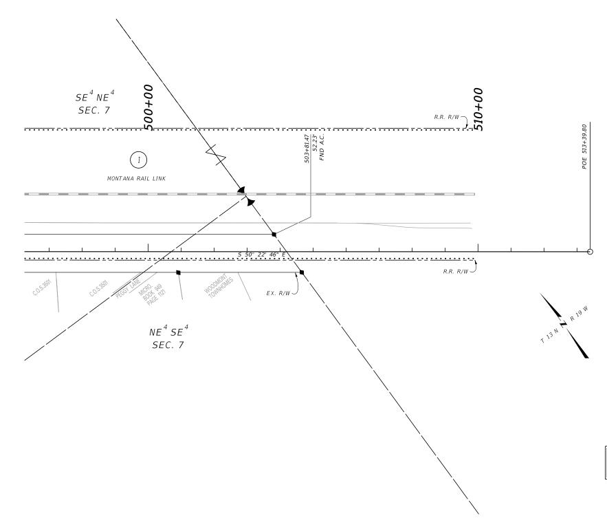
POT 504+19.76 IS 53°22'29"W 207.99' FROM THE E 1/4 CORNER OF SECTION 7. (CALC MON) POT 504+19.76 IS N3°22'29"E 2447.34' FROM THE SE CORNER OF SECTION 7. (FND 4" BRONZE CAP 59275)
